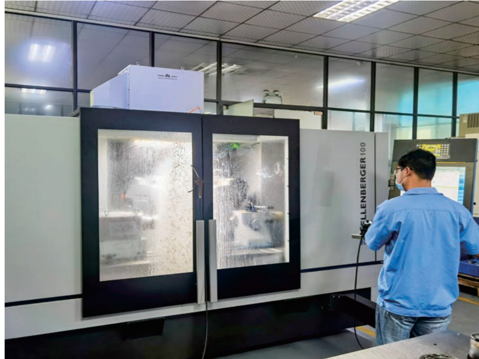
KELLENBERGER 100 — 完美的数控万能内外圆磨床 Perfect CNC universal inner and outer cylindrical grinding machine
