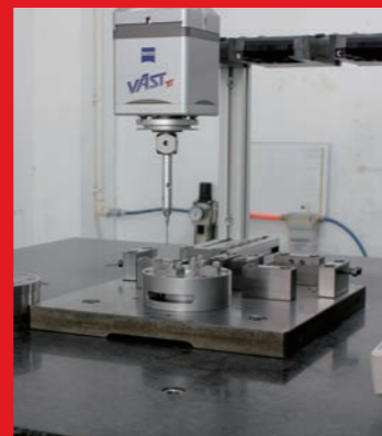
ZEISS三坐标测量仪检测 ITS卡盘 ZEISS coordinate measuring machine detects ITS Chuck
